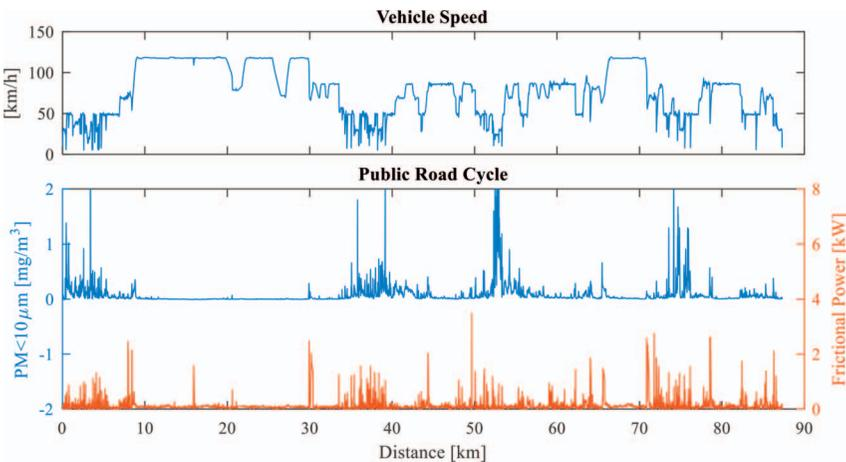
FIG. 7 — Vehicle speed, emissions values and frictional power along the public road cycle.
