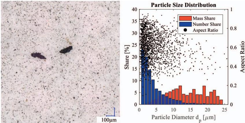
FIG. 8 — Microscopic image of TRWP sample (left) mass/number share and aspect ratio based on image processing software (right).
