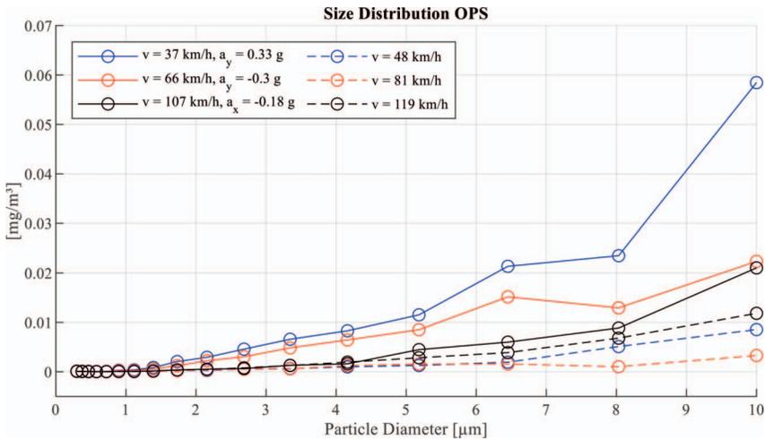
FIG. 9 — Mass-related PSD for different driving maneuvers (public road cycle) 22.
