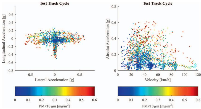
FIG. 3 — Correlation between vehicle dynamics properties and TRWP emission based on a test track cycle: influence of longitudinal/lateral acceleration and vehicle velocity.
