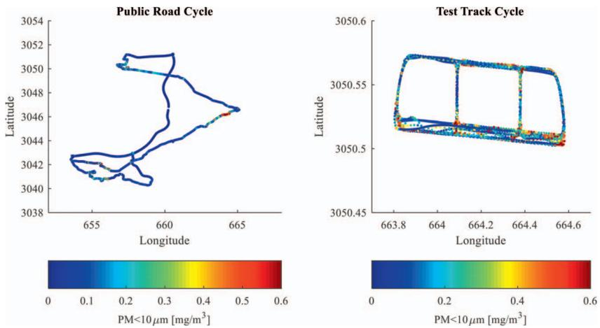
FIG. 2 — Test environments for TRWP measurement (left) public road cycle (right) test track cycle.
