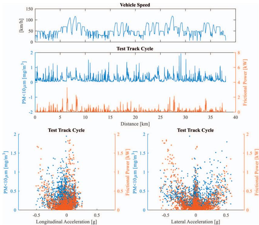
FIG. 5 — Comparison of particle concentration and frictional power as a function of longitudinal and lateral acceleration (test track cycle).
