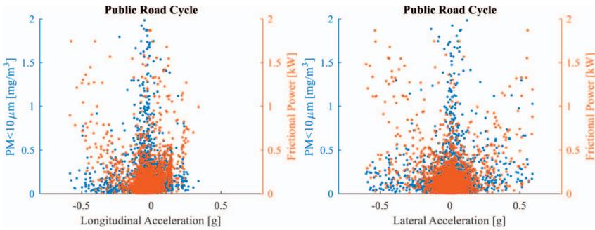
FIG. 6 — Comparison of particle concentration and frictional power as a function of longitudinal and lateral acceleration (public road cycle).
