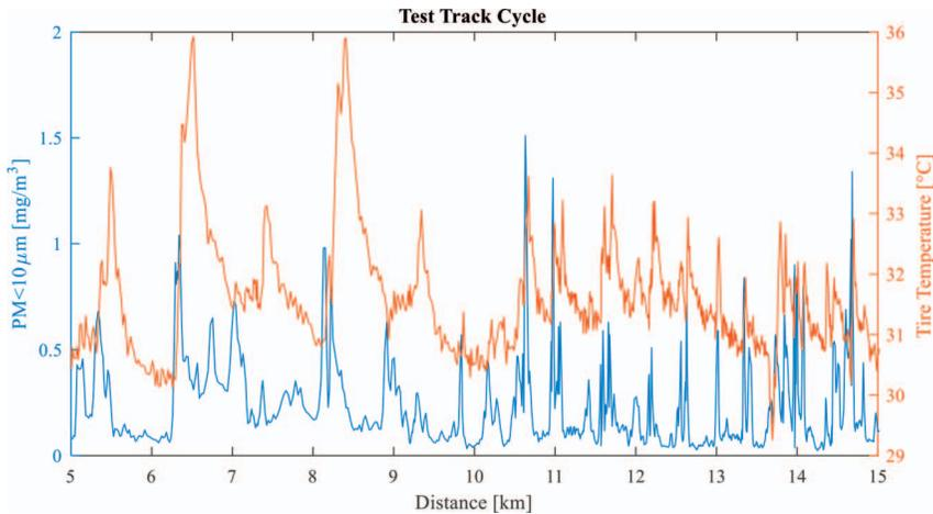
FIG. 4 — Correlation of tire temperature and particle concentration.
