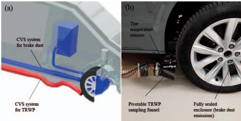
FIG. 1 — (a) CVS systems for BWP (blue) and TRWP (red) implemented into a measurement vehicle (b) pivatable TRWP inlet funnel behind the right front tire.
